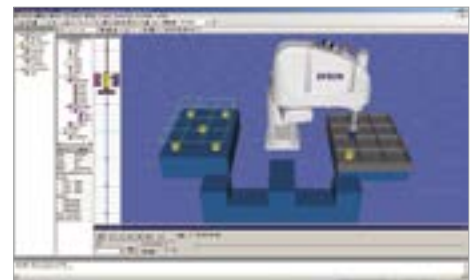
3D simulation included with Epson RC+ software
